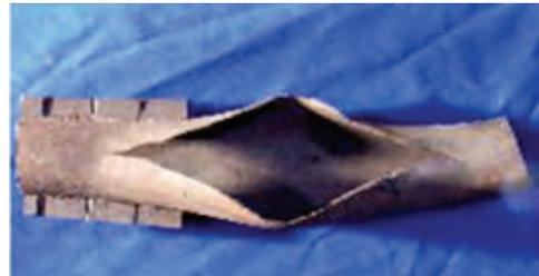
**Figure 9.2.11.** Boiler tube – failure (rupture)
