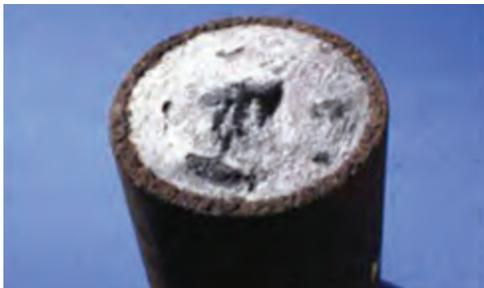
**Figure 9.2.8.** Boiler tube – scale deposit
