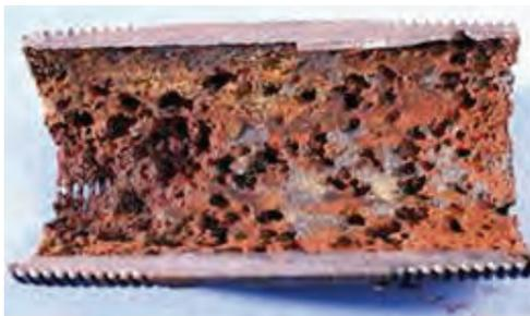
**Figure 9.2.12.** Condensate pipe – oxygen pitting
