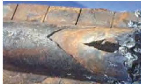
**Figure 9.2.9.** Boiler tube – failure (rupture)
