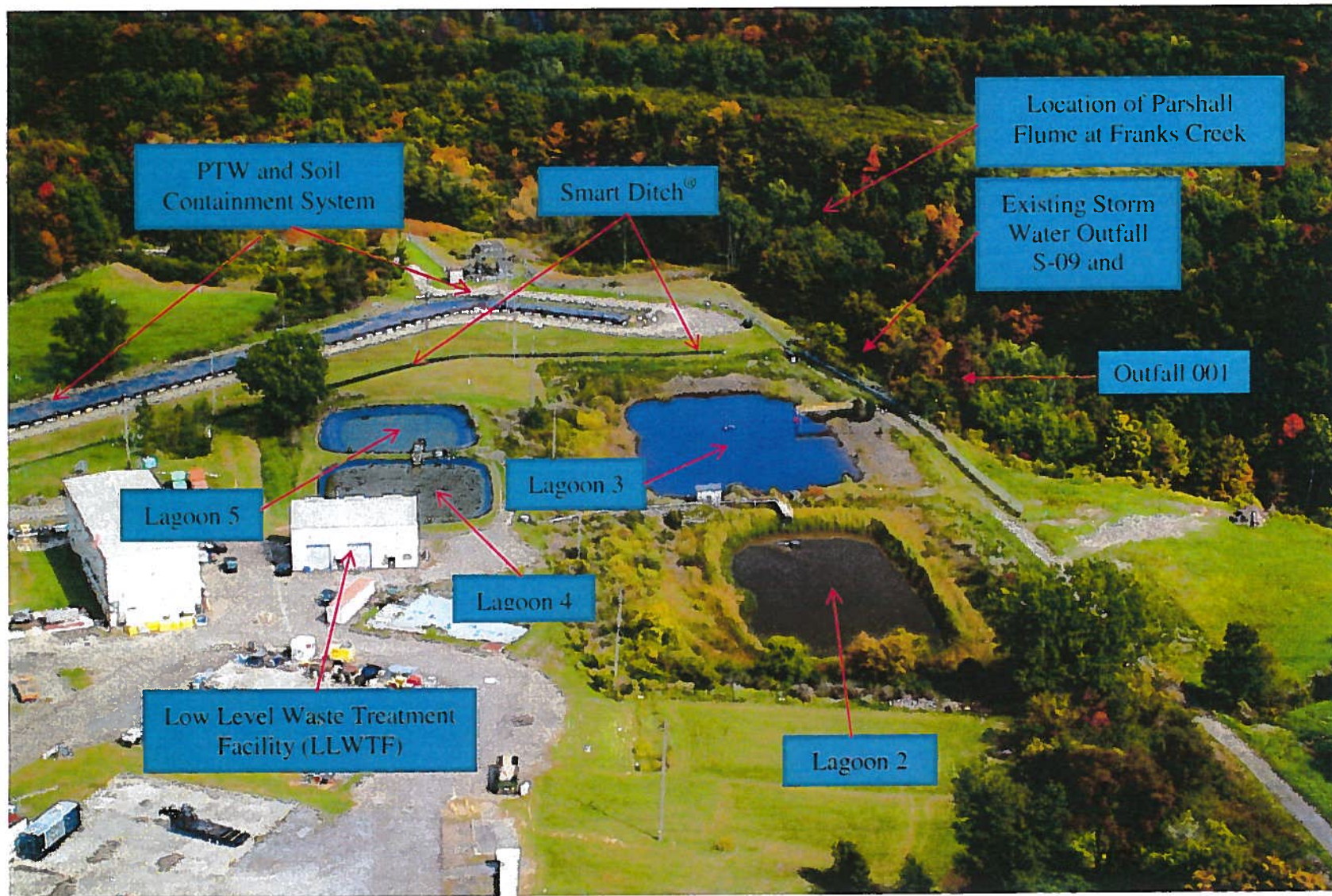
Figure 3. 2015 Aerial photograph of the West Valley Demonstration Project North Plateau depicting Smart Ditch® and Lagoons.
