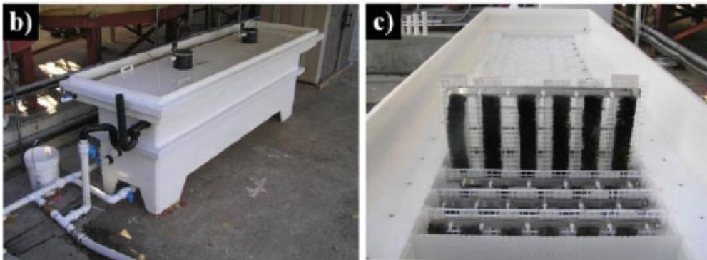
An 1000 L pilot MEC reactor treating winery wastewater and producing H<sub>2</sub>
