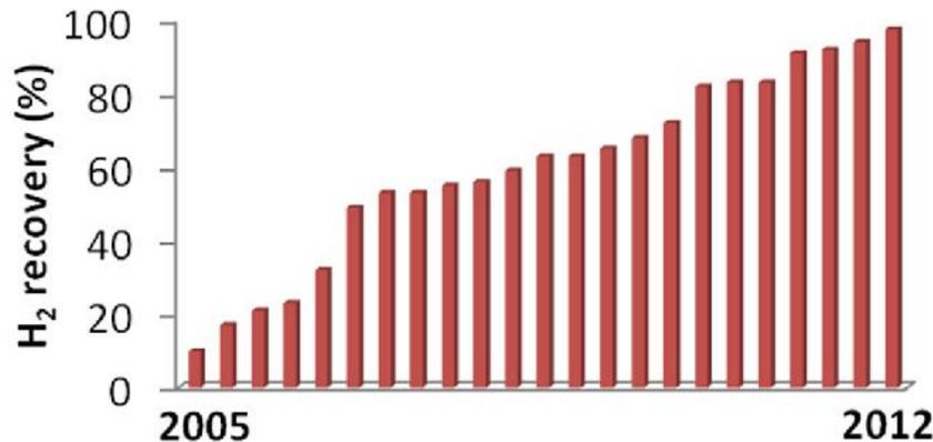
Progress on H<sub>2</sub> recovery or yield from biomass (based on 12 mol H<sub>2</sub>/mol hexose or 4 mol H<sub>2</sub>/mol acetate, etc)
