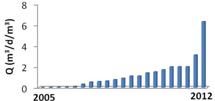
Progress on H<sub>2</sub> production rate Highest was 17.8 m<sup>3</sup> H<sub>2</sub>/m<sup>3</sup>d at 1V in a small reactor
