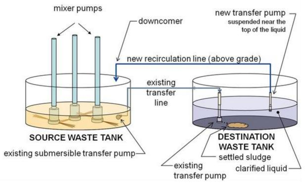
Figure 5.2-2. Recirculation Heel Removal Method
