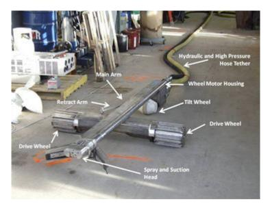
Figure 5.2-1. Mantis platform in the vendor's test facility
