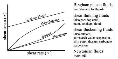
Figure 2.3-1. Stress vs. rate relationship for various fluids
