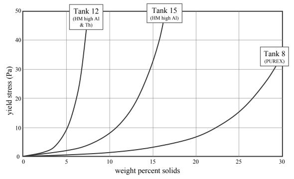
Figure 2.5-1. Yield stress vs. solids concentration for various waste tanks
