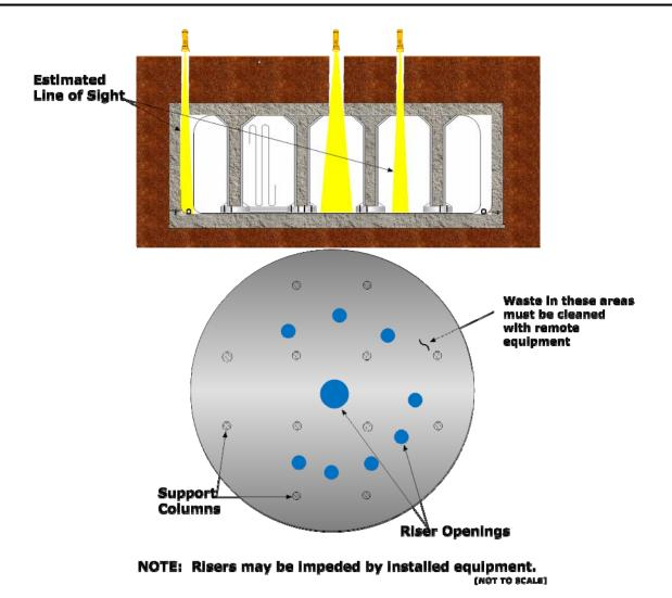
**Figure 3.2-2.** Access area for a typical Type I waste tank
