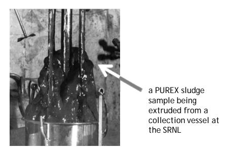
**Figure 2.3-2.** PUREX sludge sample
