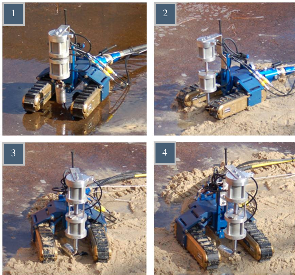
Figure 4.2-1: Waste Tank Floor Sampling Process During Mock-Up Testing
