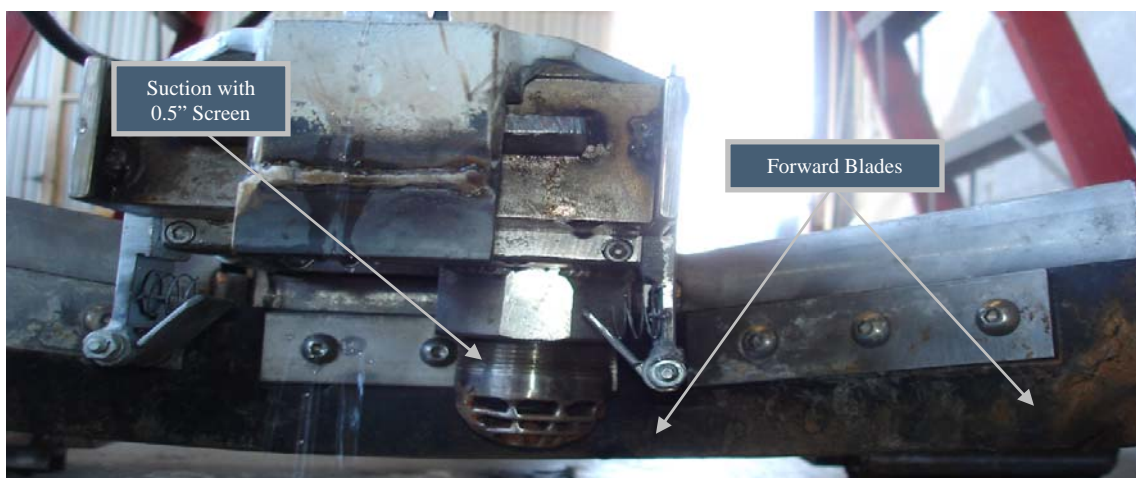
Figure 3.4-3: Mantis Suction Head Screen and Blades
