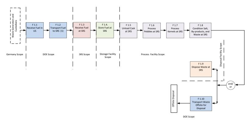
Figure 3: HTGR Functional Flow Diagram (Level 1 Functions)
