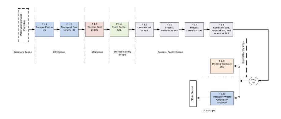
Figure 2: HTGR Functional Flow Diagram (Level 1 Functions)
