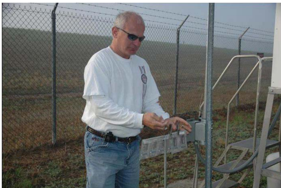
Figure 5-3 An Environmental Monitoring Field Technician Removes TLDs from the Burial Ground North Air Station
