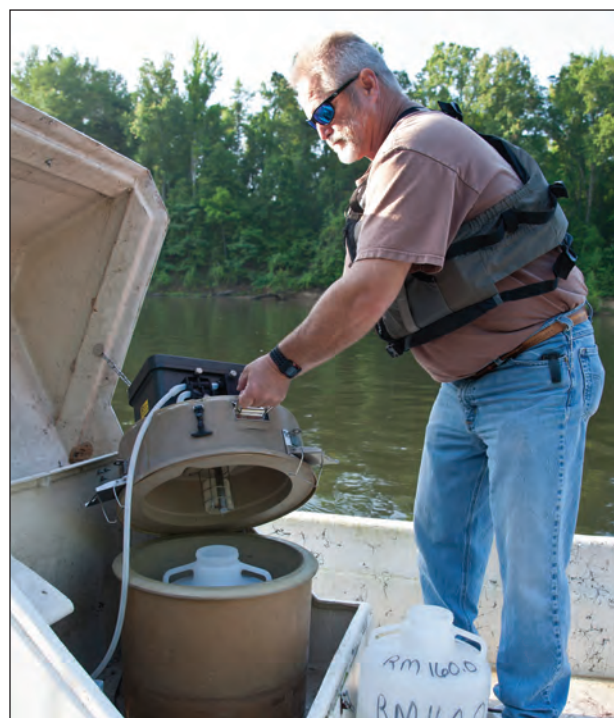
River Surveillance Sample Collection from Automated Samper at River Mile 160
