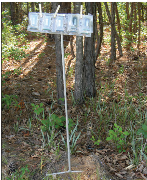
Thermoluminescent Dosimeters Placed in the Field for Ambient Gamma Exposure Monitoring
