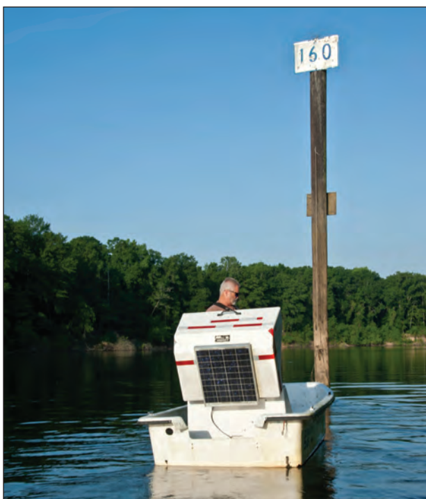
River Surveillance Sample Collection from Automated Samper at River Mile 160
