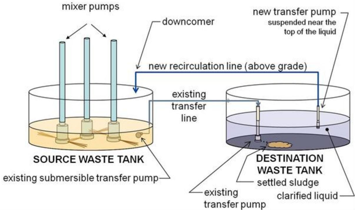
**Figure 5.2-2.** Recirculation Heel Removal Method
