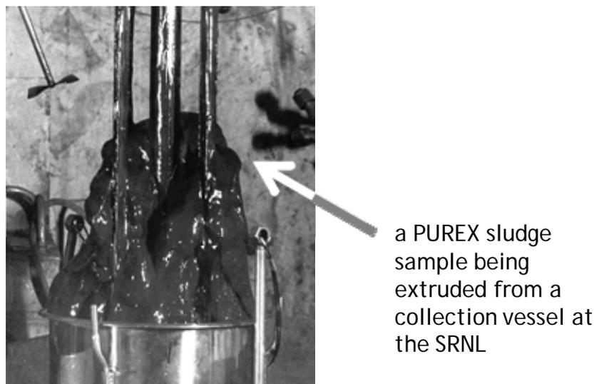
**Figure 2.3-2.** PUREX sludge sample
