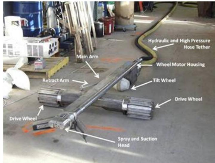
**Figure 5.2-1.** Mantis platform in the vendor's test facility
