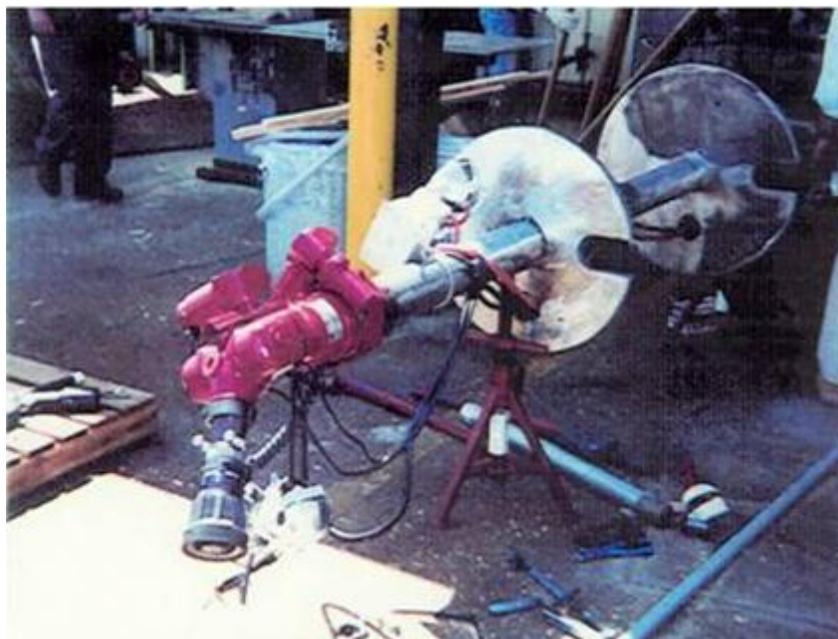
**Figure 6.3-2.** Water brush during fabrication
