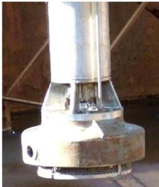
**Figure 5.1-2.** An SLP staged for trial runs at the SRS test facility
