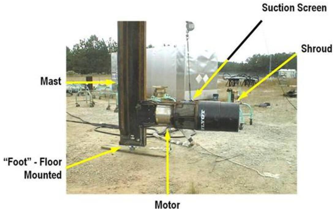
Figure 6.3-1. Tank 19 Flygt mixer at the SRS test facility
