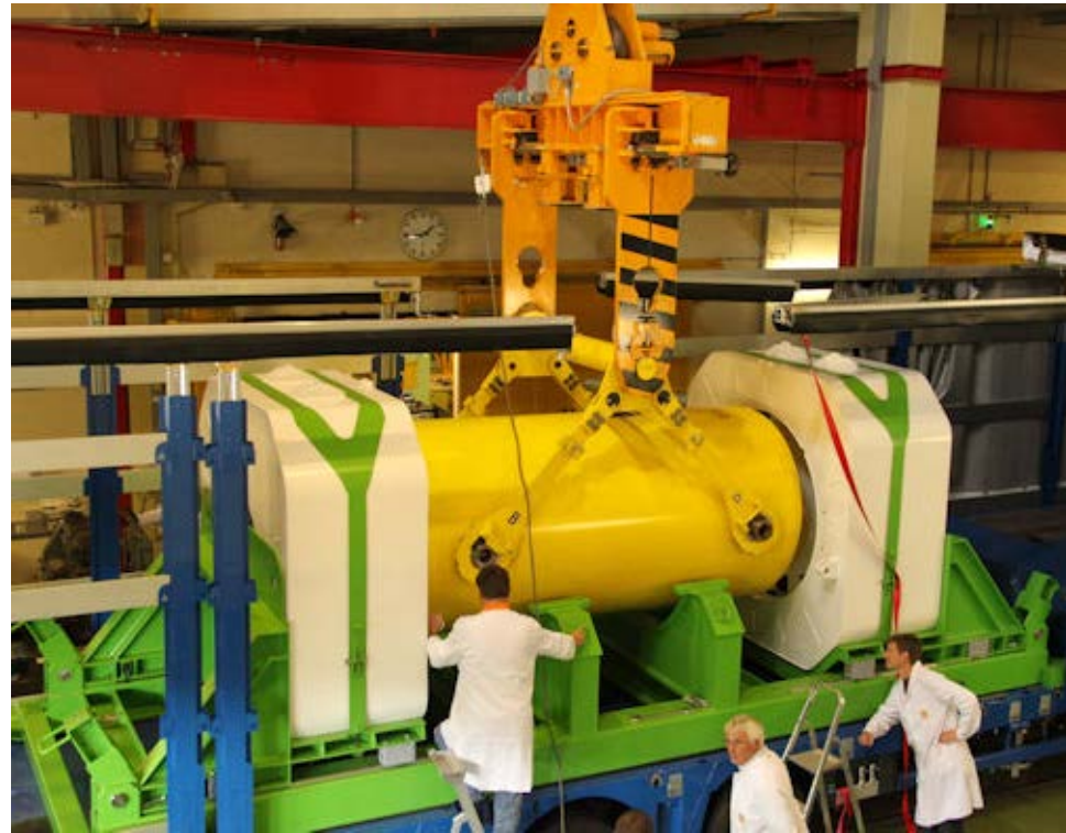
CASTOR Cask being loaded into the transportation frame
