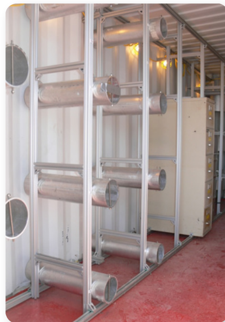
MPF "birdcage" racks ensure correct spacing of plutonium containers.
