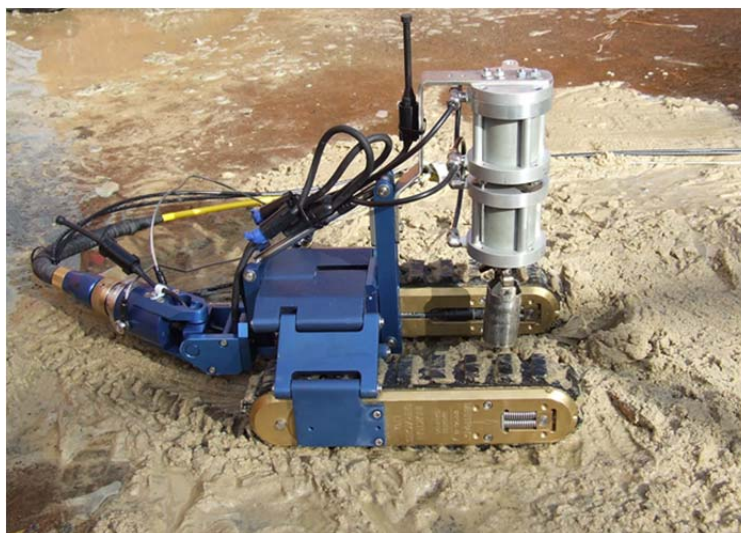
Figure 5.2-7: Robotic Sampler at Test Facility
