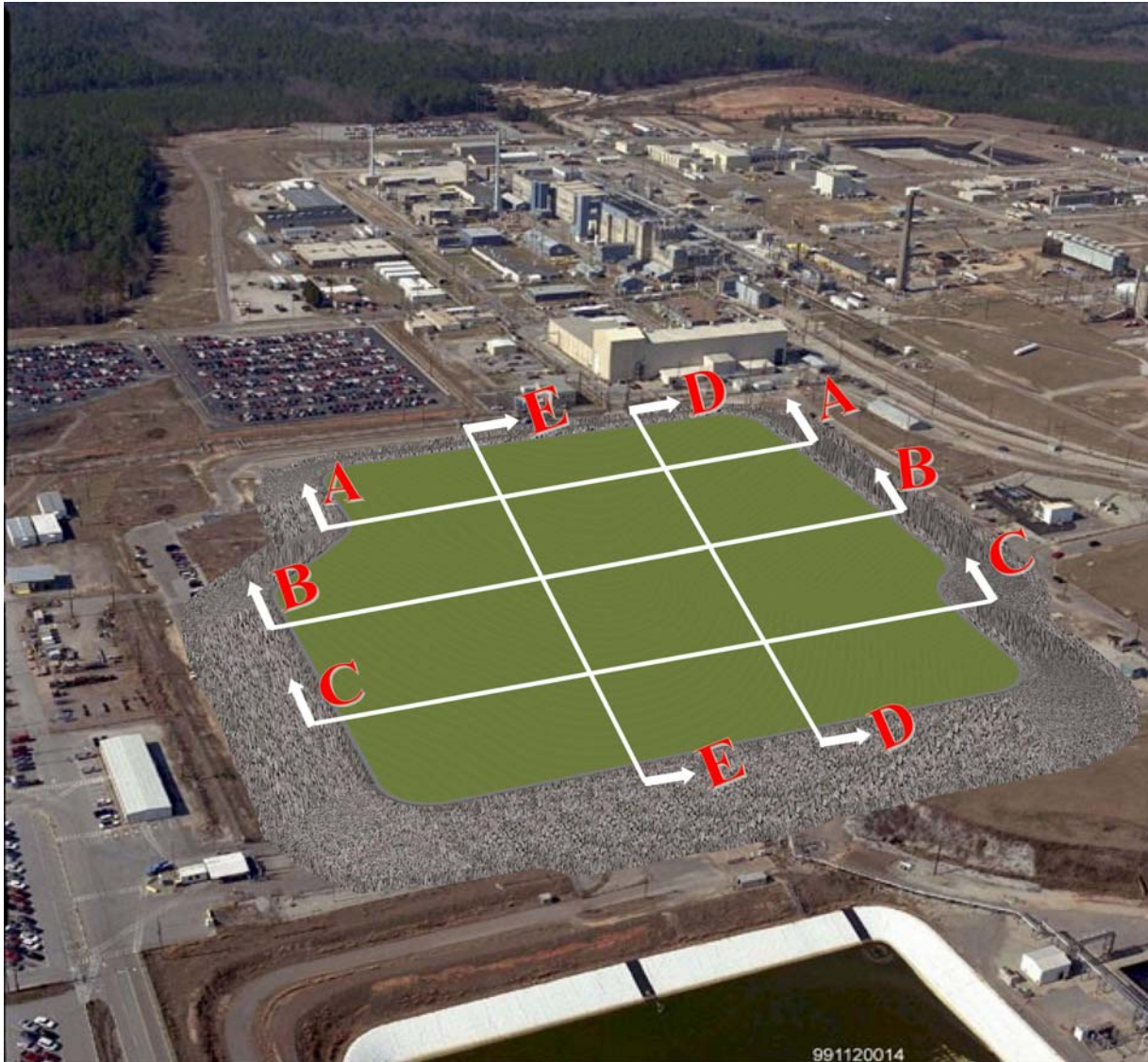
Figure 2.6-2: FTF Closure Cap Conceptual Design, Cap Footprint
