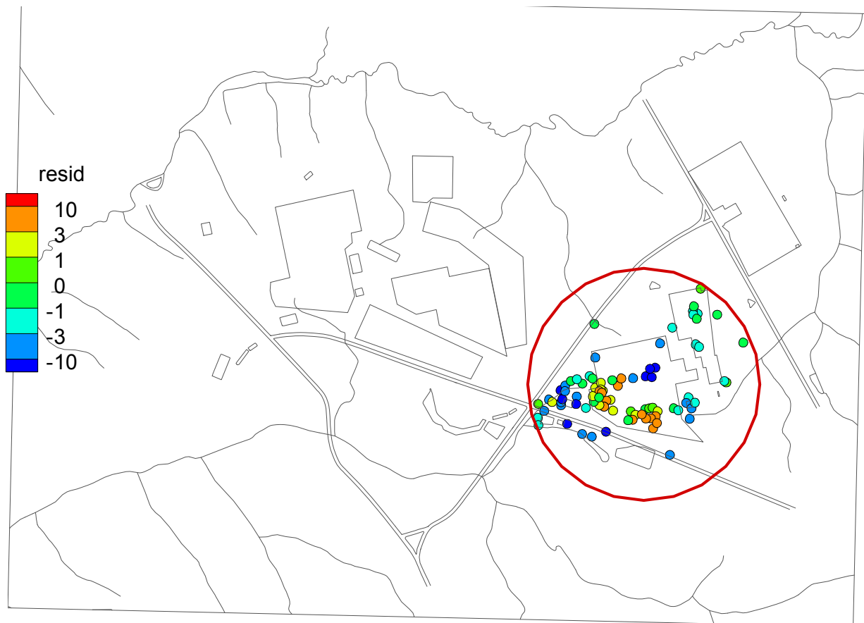
Figure RAI-FF-2.2: GSA/PORFLOW Hydraulic Head Residuals for 2003 Well Targets near H Area
