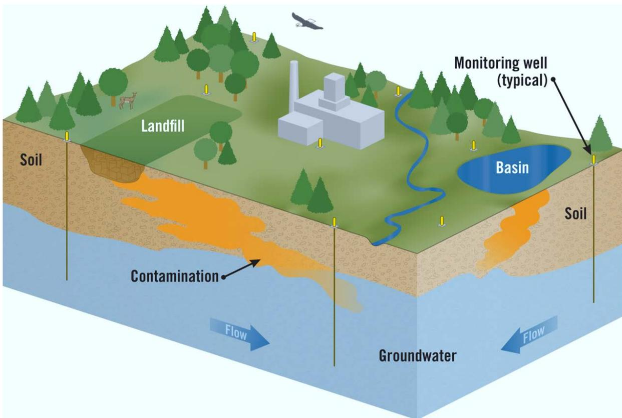
Figure 7-2 How Contamination Gets to Soil and Groundwater
