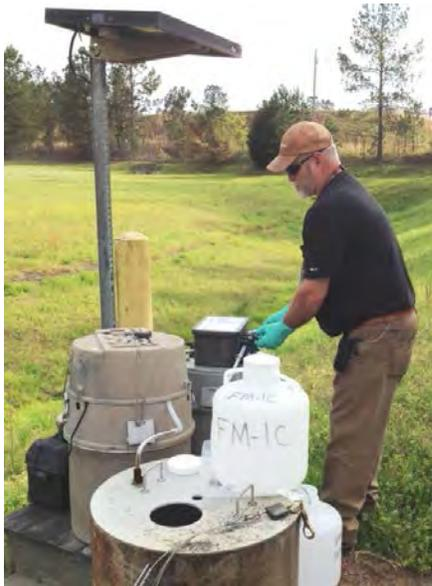
**A Field Technician Replaces Tubing for an Automated Water Sampler at a Liquid Effluent Outfall**
