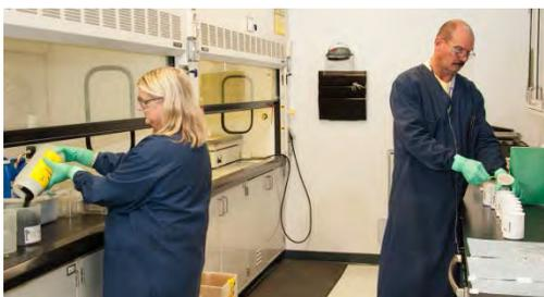
**SRS Laboratory Technicians Prepare Air Effluent Samples (filters and charcoal) for Analysis**
