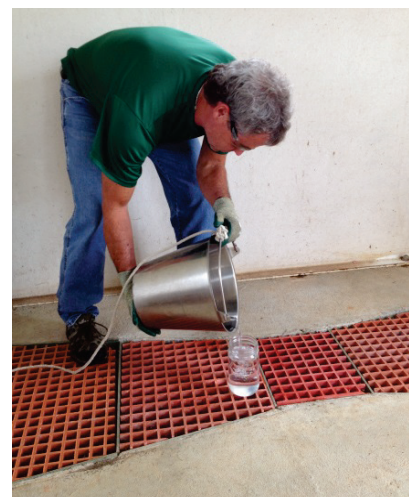
Figure 4-8 Field Technician Collects a Compliance Sample at an Industrial Wastewater Outfall
