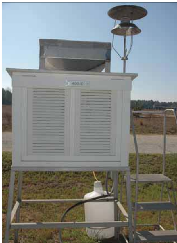
Internal (L) and External Configurations of an Air Surveillance Sampling Station
