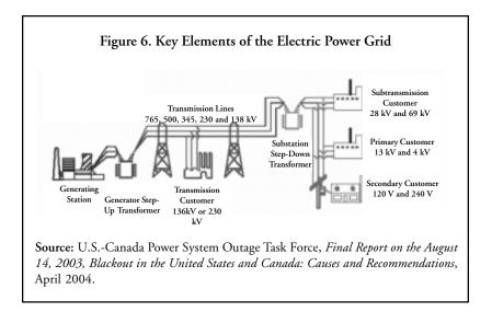
voltages in order to transmit it over the AC power system, and then "step down" voltages as it reaches customers. These transformers are a critical part of the transmission system.
