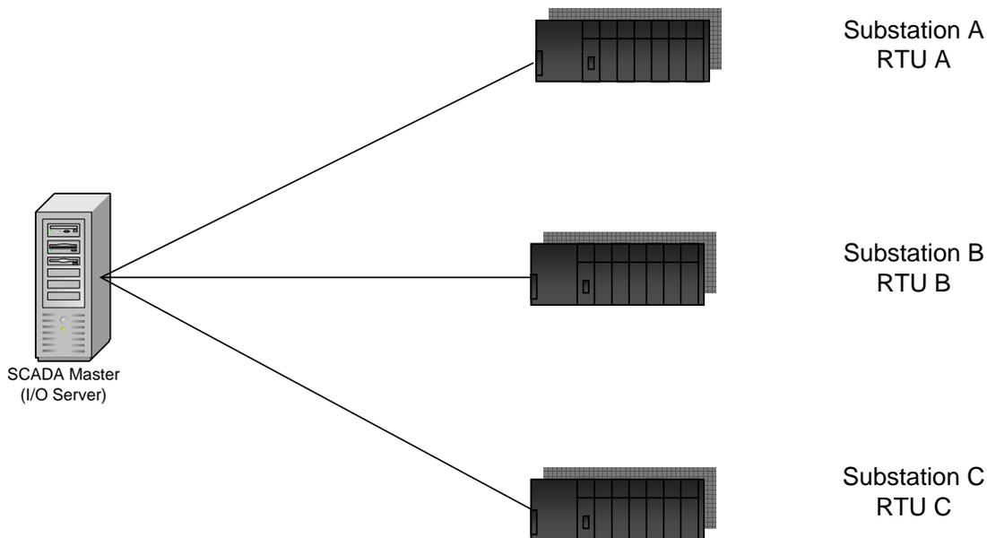
In this round-robin telemetry scheme, the Master first polls Substation A. After receiving the response from Substation A, Substation B is polled. Likewise, after the response is received from Substation B, Substation C is polled. After the response from Substation C is received, the process is repeated.
