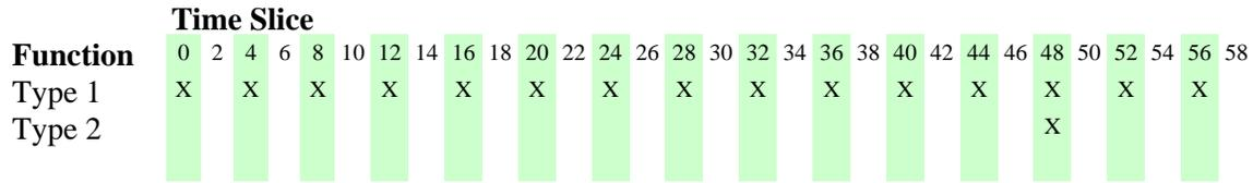
In a round-robin telemetry scheme, information from each remote device is requested in sequence and is depicted in the following diagram.
