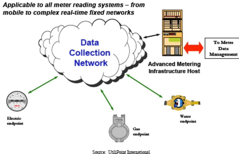
**Figure B1: Typical AMI Architecture**
