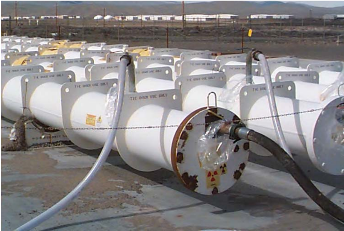
Figure 2.15. Treatment by Macroencapsulation at the LLBGs
