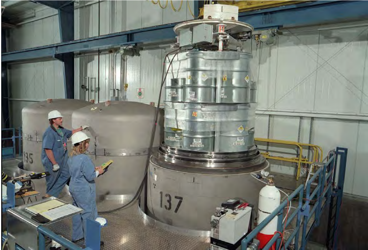
Figure 2.9. Transuranic Package Transporter-II Being Loaded in the Waste Receiving and Processing Facility
