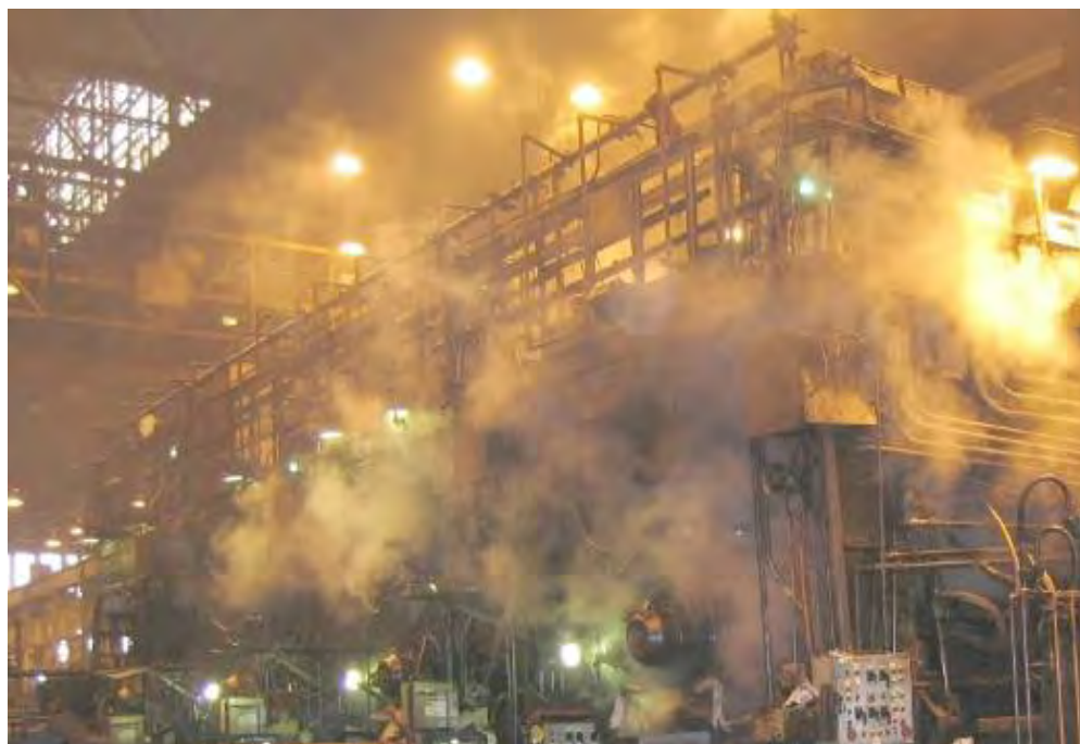
Figure 2.4: Current Tandem Mill While Operating
