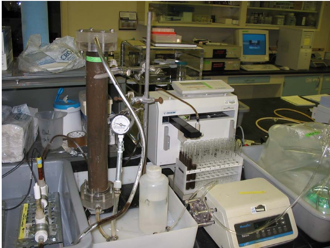
Figure 8. Column Test 3. Experimental apparatus. Tubes in fraction collector contain effluent from the NaOH injection; note the deep brown color due to humic material.
