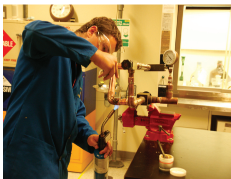
Physics undergraduate student, Zackary Rehfluss, assembling a pumping system for a dilution refrigerator in the laboratory of Professor Brian Maple at UC San Diego. The dilution refrigerator will be used to cool high pressure cells down to millikelvin temperatures for electrical transport and magnetic measurements on f -electron materials at high pressures into the megabar range.
