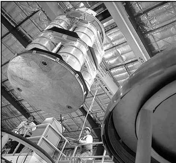
A group of 14 drums of transuranic waste at INEEL being lowered into a Trupact-2 shipping cask
