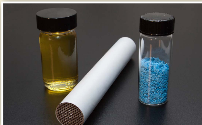
A “monolith” reactor for reforming hydrocarbon-based fuels. The reactor is created by depositing NETL’s novel pyrochlore catalyst on a honeycombed alumina structure. The catalyst converts heavy hydrocarbons, such as diesel and coal-based fuels, into hydrogen-rich synthesis gas for use in fuel cells and other applications.
