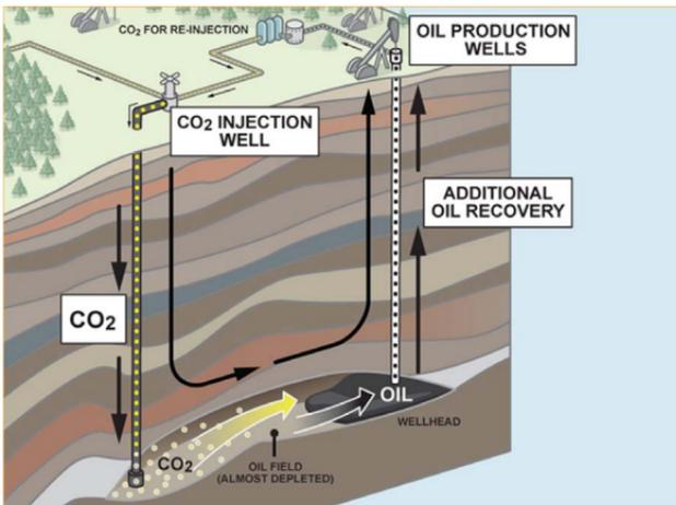
*EOR is a way to recover additional domestic oil resources from older fields and permanently store carbon dioxide underground. (Illustration: Clean Air Task Force, available at: [http://www.coaltransition.org/pages/carbon\\_storage/30.php](http://www.coaltransition.org/pages/carbon_storage/30.php).)*
