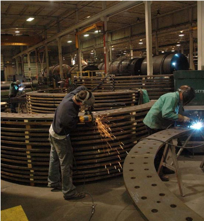
Bassett employees work on embedment (anchor) rings for the wind turbine foundations. Bassett just received a 48C tax credit to invest in capital equipment for wind turbine tower manufacturing. Photo courtesy Bassett Mechanical
