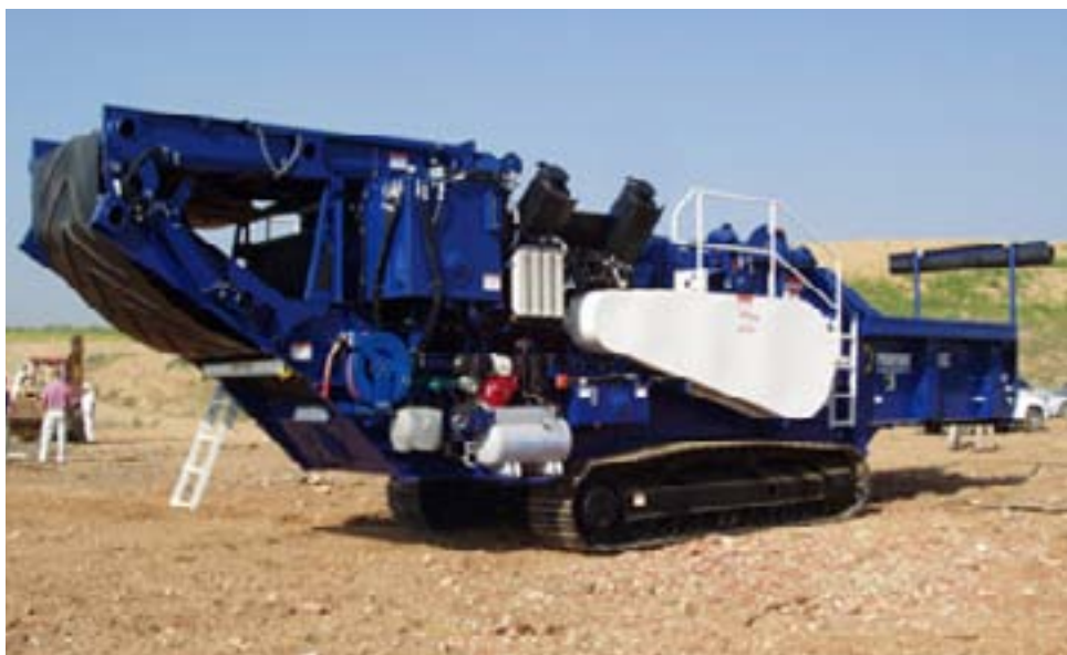
Montgomery's horizontal grinder has normal handling capacity of 108 tons per hour. | Photo Courtesy of Lynda Wool
