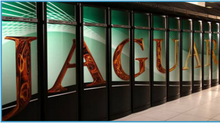
The Jaguar supercomputer, located at the Oak Ridge National Laboratory Leadership Computing Facility, can perform 700 trillion calculations per second and is the world's most capable scientific computing resource.
