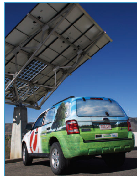
Converted Ford Escape PHEV charging from a photovoltaic system as part of a National Renewable Energy Laboratory electric-vehicle grid-integration project.
