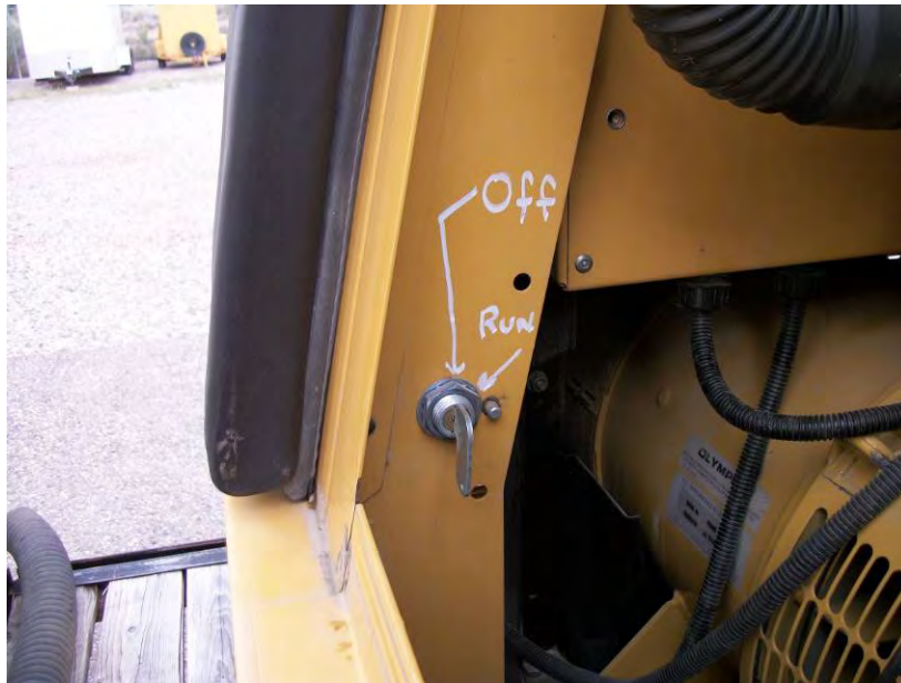
Figure 2. Battery Isolation Switch
