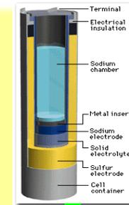
Traditional tubular Na – sulfur cell, operated >300-350°C
