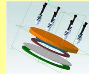
Newly developed planar sodium metal-halide cell, operated <250°C
