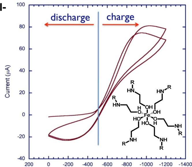
Potential (mV vs Ag/AgCl, BMICl in EMI-Im)
