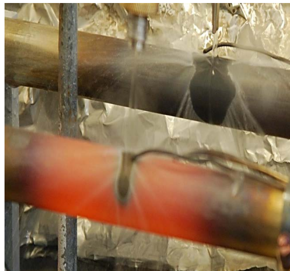
Figure 3.7. Thermal Fatigue Setup Operation. The upper sample has cooled below the visible thermal temperature while the lower sample has just started the cooling cycle and is still red hot. The shape of the water jets can be seen in this photo, most clearly for the upper sample.
