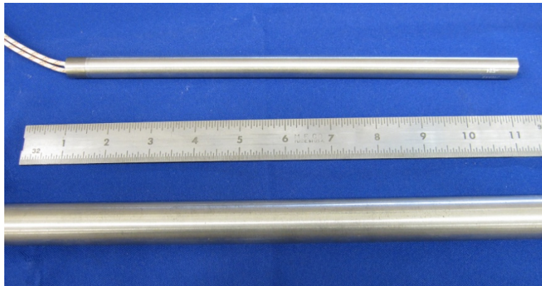
Figure 3.5. Example of Tubular 304SS Specimen and Cartridge Heater
