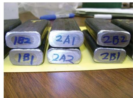
Figure 1. Coupons cut from the extruded bars. Note that the inner portion is the NFA, and the outer rim is the carbon steel can.
