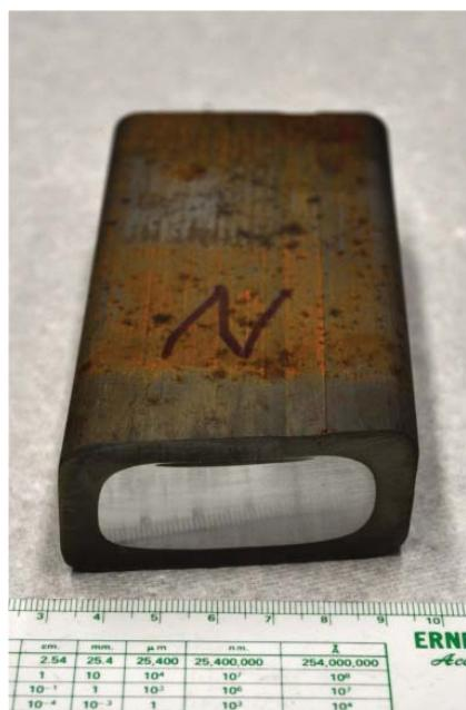
Figure 1. A 2.4-kilogram extruded bar of 14YWT advanced ODS alloy.
