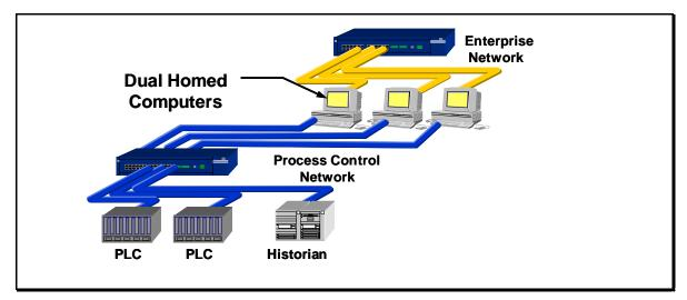
Figure 2: Network Separation Using Dual-Homed Computers
