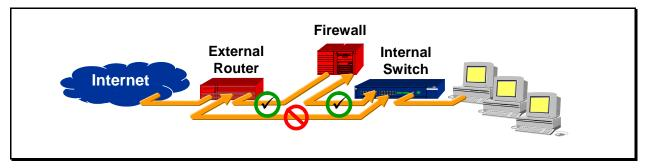
Figure 6: Network Separation with Firewall/Router Combination (Internet Example)
