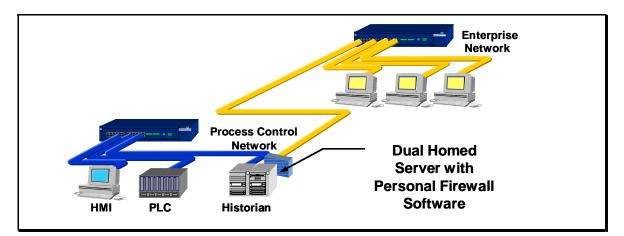
Figure 3: Network Separation Using Dual-Homed Server with Personal Firewall Installed
