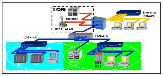
Figure 9: Firewall with Demilitarized Zone and SCADA/PCN VLANs
