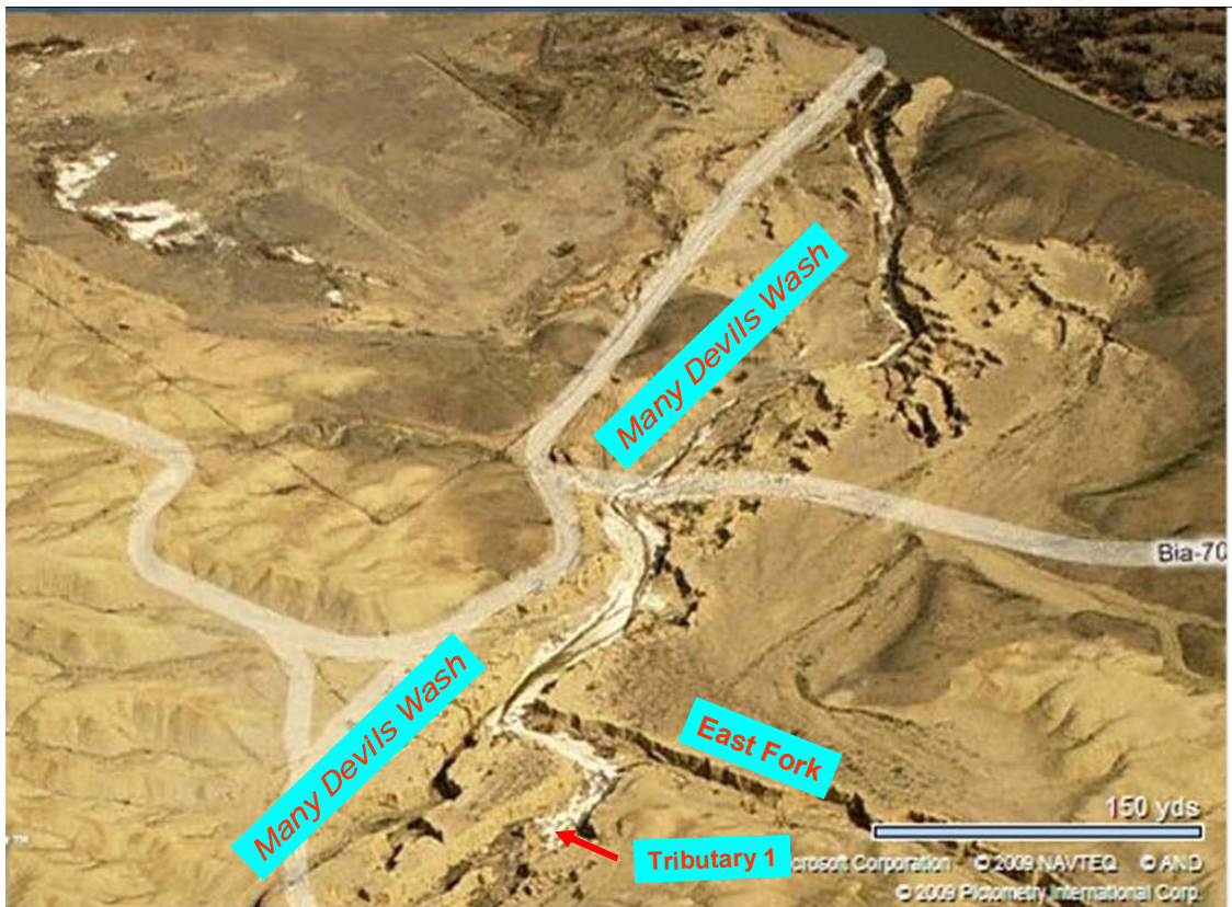
Figure 6. Oblique Air Photo of Project Area Showing Efflorescence Extending from Tributary 1 to the Mouth of Many Devils Wash (Farthest upstream efflorescence is at the tip of the Tributary 1 arrow. Photo base is from the Microsoft Bing website.)
