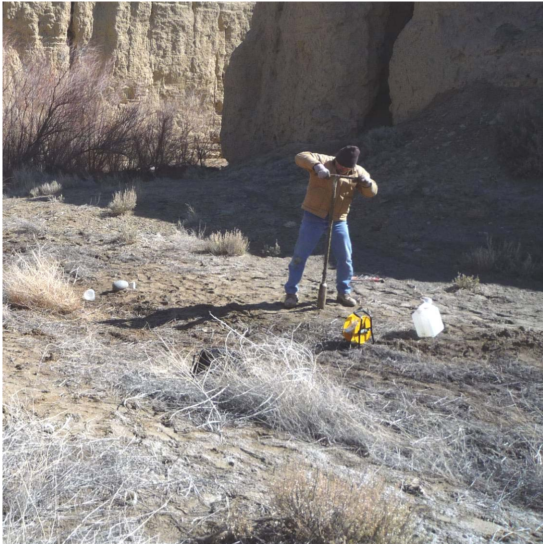
Figure 14. Sample Point Being Installed in Tributary 1 Using Hand Coring Device
