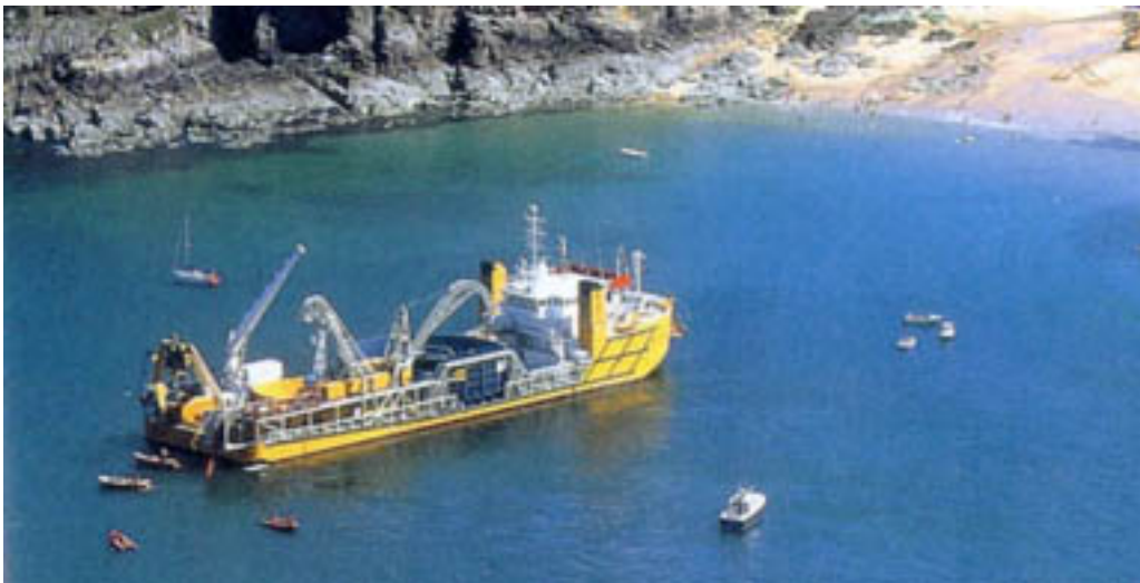
Figure 2-3 Typical Cable Laying Ship
