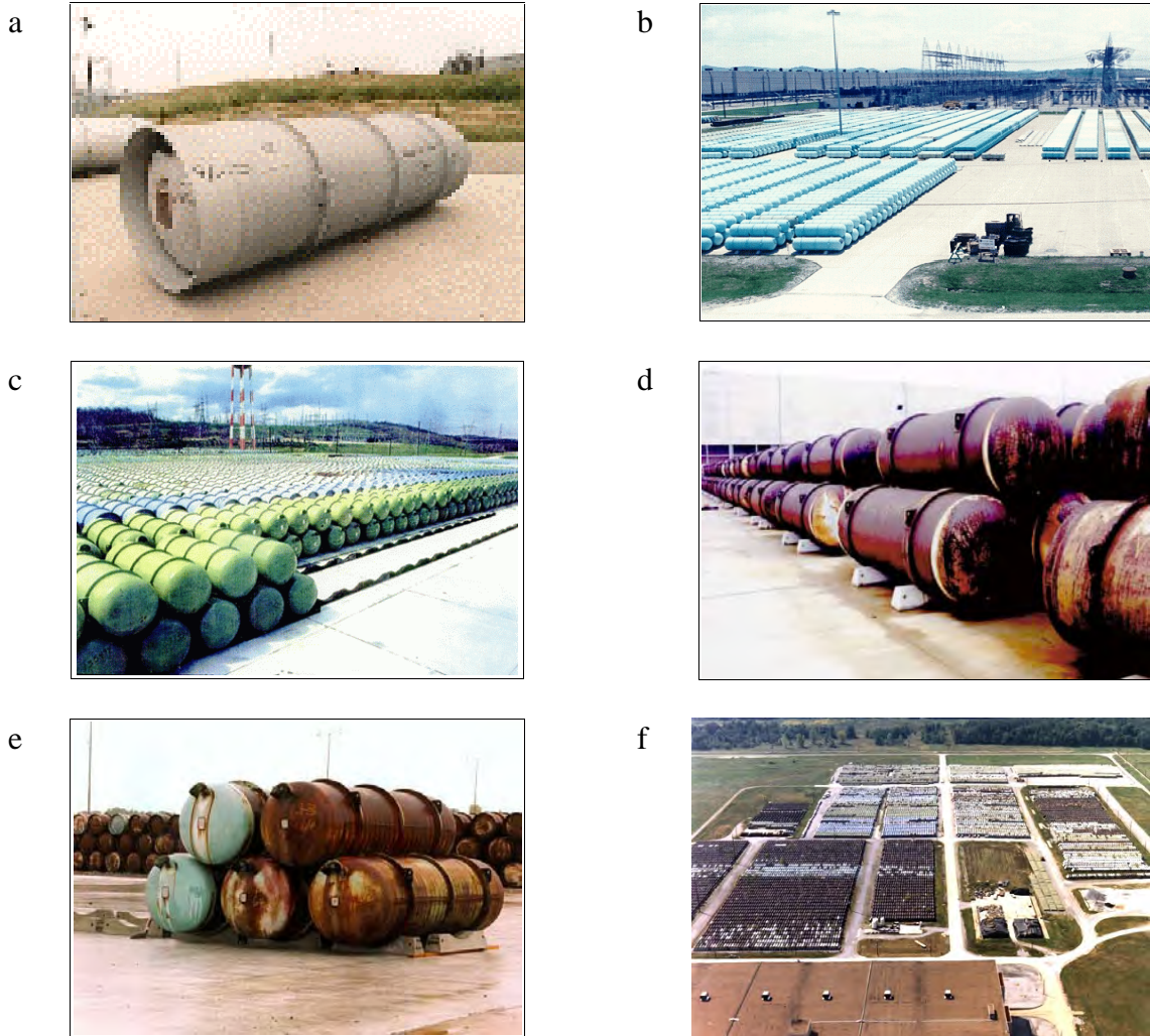
FIGURE 1.1-1 Storage of DUF 6 Cylinders: (a) Typical 14-ton (12-t) skirted cylinder. (b) New cylinder storage yard at the Paducah site. (c, d, e) Cylinders stacked two high on concrete chocks. (f) Cylinder yards at the Paducah site.
