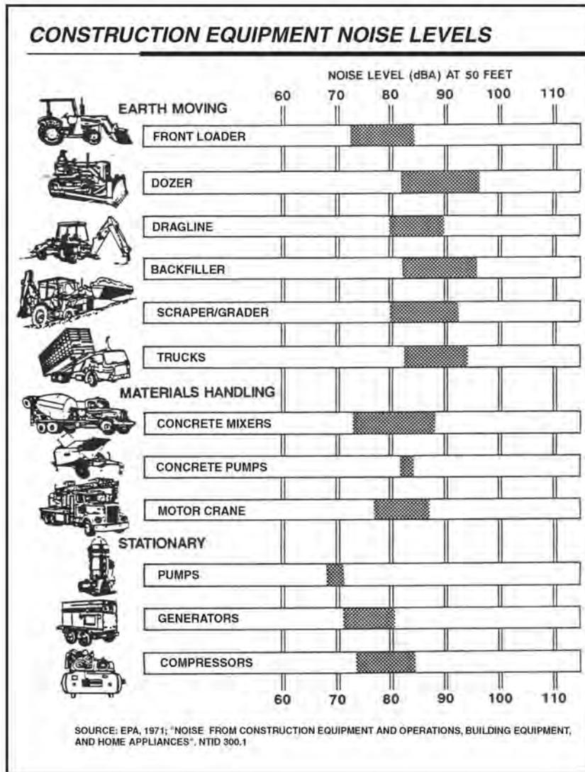
Figure 3-8. Typical Construction Equipment Noise Levels
