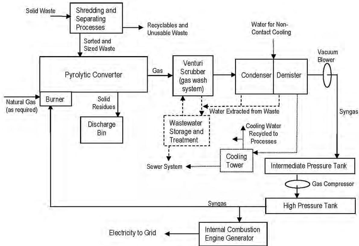
**Figure 2-3. Simplified Schematic of Oneida Energy Recovery System Process Elements**
