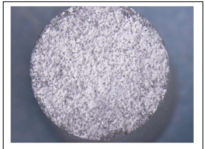
Figure 3. Cermet (\text{Pu}_{0.73}\text{Th}_{0.23})\text{O}_2/\text{Mo} (40:60 vol%) pellet end face.
