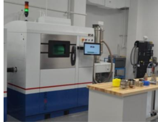
Eaton L-PBF printers: EOS M290 and Concept Laser M2 UP1
