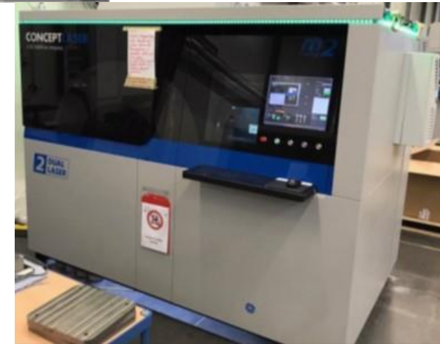
Eaton L-PBF printers: EOS M290 and Concept Laser M2 UP1
