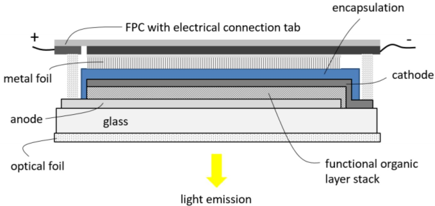
Figure 1 - schematic illustration of the LumiCurve Wave
