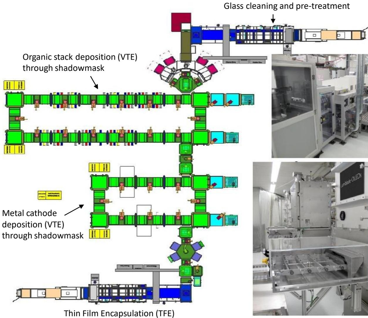
G2.5 production line capable of 2-6 stack OLEDs with 40+ organic layers
