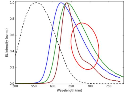
**Figure 4:** Normalized bottom emission device EL spectra for an advanced narrow deep red emitter (red) vs. a conventional red (blue) and the same emitter red-shifted to the peak wavelength of the narrow emitter (green). The photopic response function (black, dashed) is also shown.
