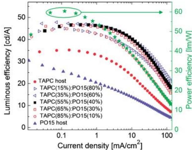
FIG. 3. (Color online) Luminous efficiency roll-off characteristics for devices with varying mixed host composition. The OLED with 55 wt % TAPC:40 wt % PO15 mixed host was considered the optimized device with respect to a combination of low operation voltage and stable roll-off. Hence, the representative power efficiency for the optimized device is included (solid stars).
