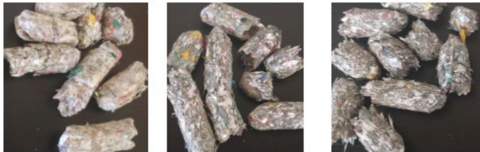
Durable 12mm pellets produced at varying paper:plastic ratios
