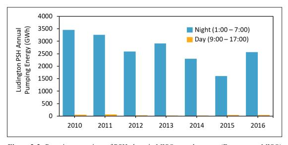
Figure 2-3. Pumping operations of PSH plants in MISO over the years. (Data source: MISO)
