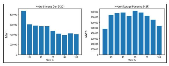
Figure 2-5. PSH generation and pumping relative to wind generation. (Data source: MISO)
