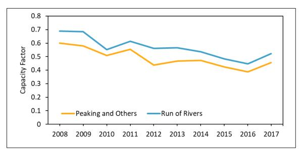
**Figure 2-11.** Capacity factors of conventional hydro resources in ISO-NE. (Data source: FERC Electric Quarterly Report [EQR])
