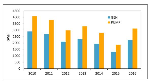
**Figure 2-23**. Annual generation vs. pumping load for PSH resources in MISO. Total generation and pumping have decreased since 2010. (Data source: MISO)
