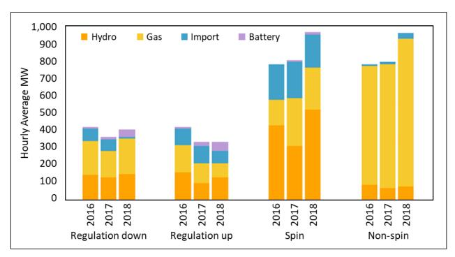
**Figure 2-15**. Contribution of hydropower resources for essential reliability services in CAISO.<sup>21</sup> Hydropower's total capacity ranges from 10–15% of total capacity in CAISO. (Data source: CAISO)
