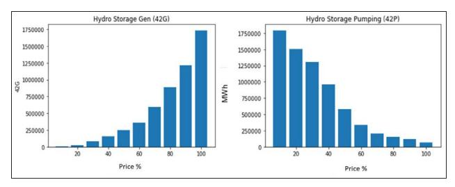
**Figure 2-7**. PSH generation and pumping relative to system prices (LMPs). (Data source: MISO)
