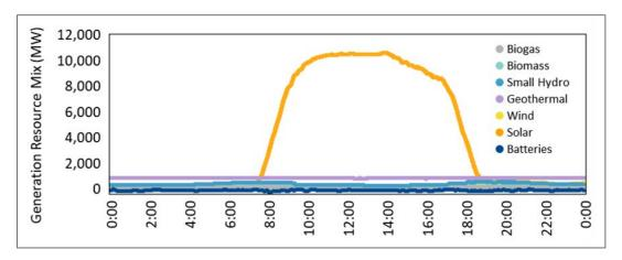
Figure 2-30. The generation mix (MW) on March 18, 2019 in CAISO. (Data source: CAISO)
