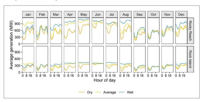
**Figure 2-18**. Comparison of average hourly generation during dry, average, and wet years at Rocky Reach and Rock Island Dams. During spring and early summer months of wet years at both Rocky Reach and Rock Island, the flexibility of operations is restricted due to high flow conditions. (Data source: Chelan PUD)
