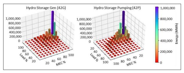
**Figure 2-8**. Comparison of PSH operations in pumping vs. generation modes in MISO (2015–2017). Marginal Energy Charge (MEC) is the energy component of the LMP. (Data source: MISO)
