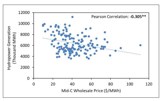
**Figure 2-21**. Hydropower generation is negatively correlated with Mid-C wholesale price. (Data source: EIA)
