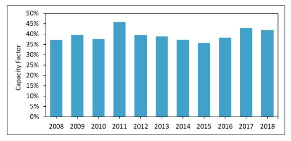
Figure 2-10. Capacity factor of conventional hydropower resources in the US. (Data source: EIA)
