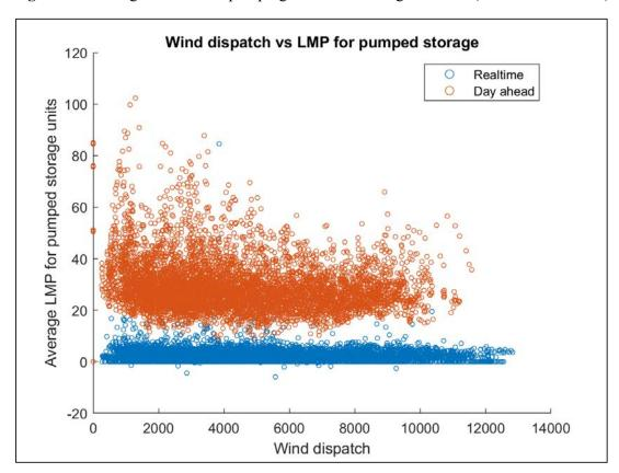
Figure 2-6. Wind generation does not affect LMPs at the PSH locations in MISO. (Data source: MISO)
