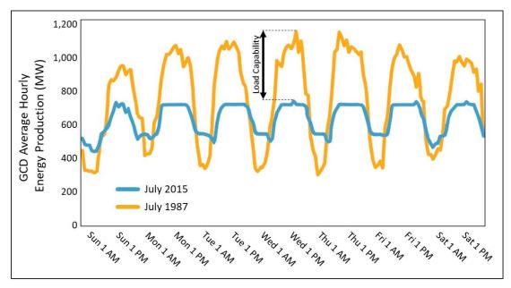
**Figure 2-17**. Hourly energy production at the GCD powerplant during a July week in 1987 and 2015. Flexibility was restrained with the implementation of new environmental restrictions.
