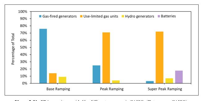
Figure 2-31. FRA capacity provided by different resources in CAISO. (Data source: CAISO)
