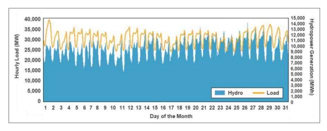
Figure 2-9. Typical pattern of hydropower operations in the Pacific Northwest compared to gross load in March 2016. Hydropower is continuing to operate in gross load-following patterns as designed. (Data source: EIA)
