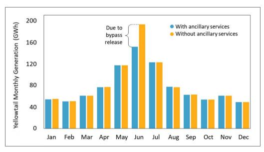
Figure 2-29. Monthly projected generation for Yellowtail hydropower facility during a sample year.
