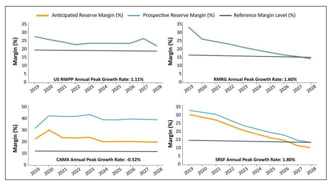
Figure 2-13. Capacity RMs between 2019 and 2008 in the four NERC subregions.
