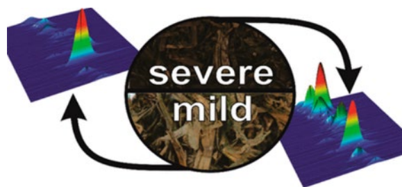
Figure 6. Two-dimensional gas chromatography/mass spectrometry is used to track the impact of degradation during storage on hemicellulose content and composition.
