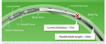
High-energy-capture machines with highly flexible blades open many more parts of the United States to wind development by solving logistical and science challenges associated with these machines.
