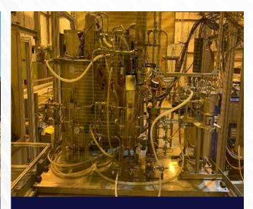
Completed installation of the caustic dissolver assembly which supports the recovery of plutonium 244 at the Savannah River Site.
