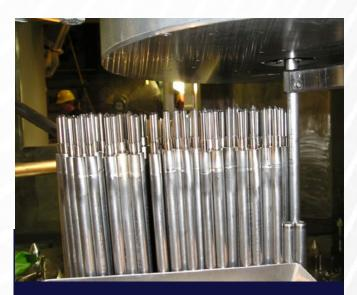
Tritium: Completed irradiation of 1,584 tritium-producing burnable absorber rods (TPBARs) in Fuel Cycle 16 in May at Watts Bar Unit 1 in Tennessee and commenced irradiation of 1,792 TPBARs in Cycle #17 at Watts Bar Unit 1 in June.
