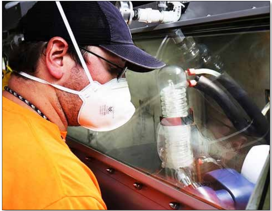
Employees, known as fissile material handlers, use shielded gloveboxes to dissolve U-233 into a low-level form so it can be mixed with grout for safe transportation and disposal. Removing the remaining inventory of U-233 at ORNL is EM's highest priority.
