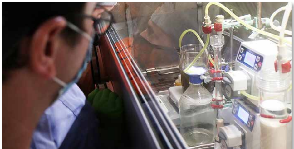
Employees, known as fissile material handlers, use shielded gloveboxes to dissolve U-233 into a low-level form so it can be mixed with grout for safe transportation and disposal. Removing the remaining inventory of U-233 at ORNL is EM's highest priority.
